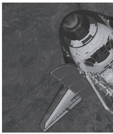
Columbia was destroyed by a complex sequence of faults relating to carrying a tank of cryogenic fuel strapped to the spaceplane's belly; falling ice damaged fragile heatshield tiles during the launch.
